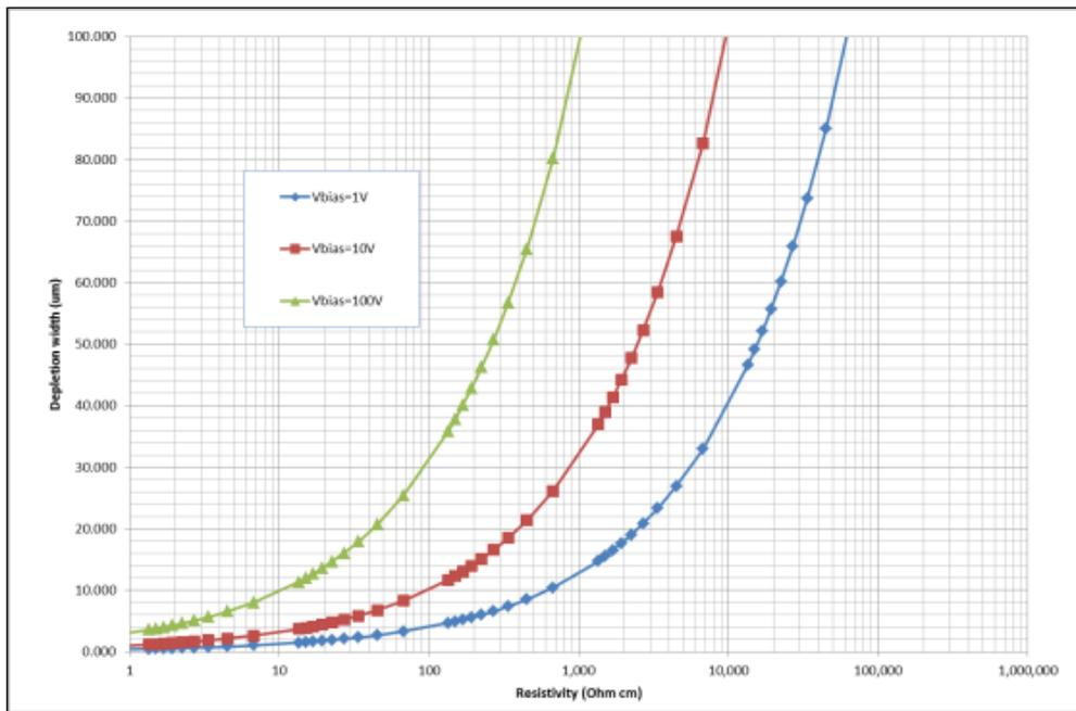
Figure 1. Calculated depletion width as a function of the substrate resistivity for different values of the applied bias voltage.
